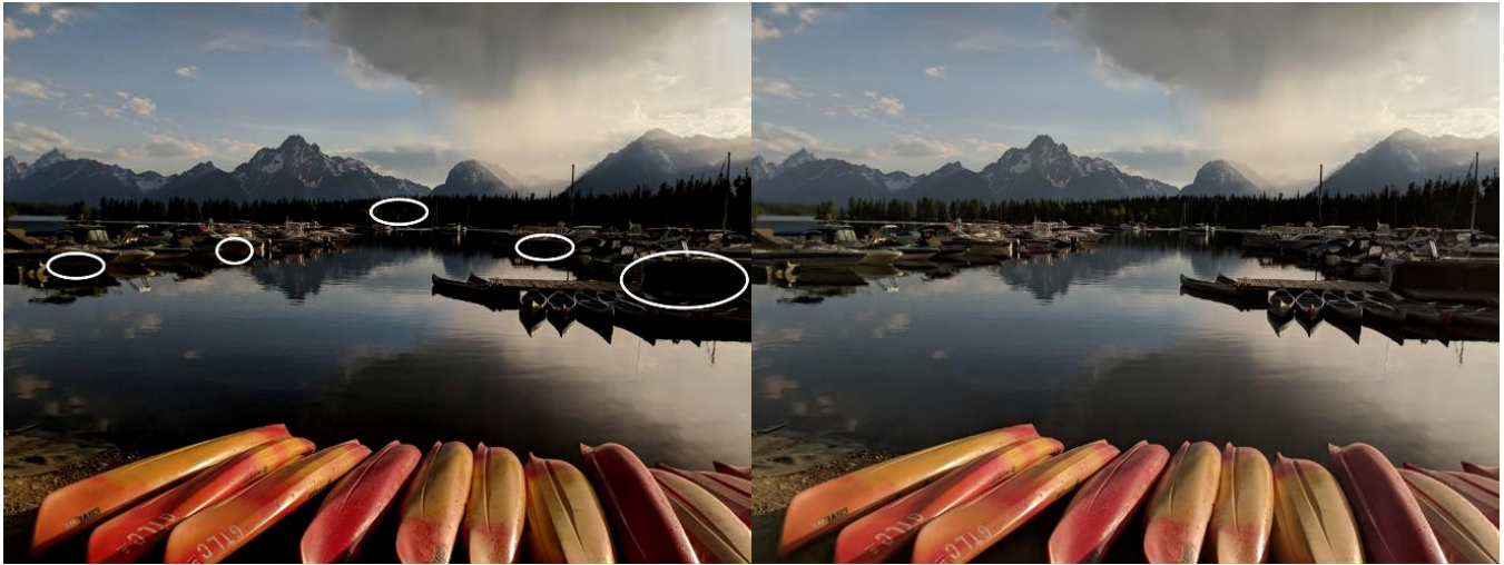
In the simulated SDR image at left, the circled shadow areas are “crushed.” The simulated HDR image at right retains significant detail in the boats, pine trees and the dock.
