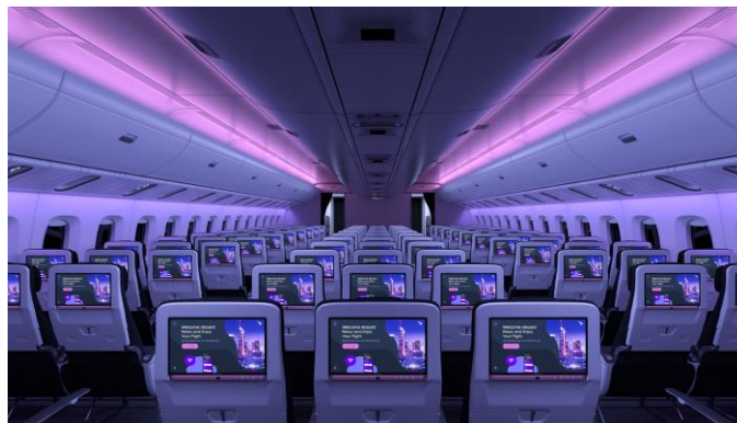
HDR10+ is implemented in the Astrova inflight entertainment system from Panasonic Avionics.
